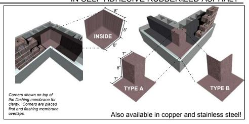
Lay drip edge in a bead of caulk first, then all preformed corners and end dams, then the roll flashing. Recess the flashing 1" from the vertical face of the masonry wall.
